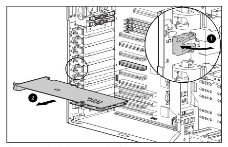
Figure 2-29. Removing the Smart Array 3200 Controller
